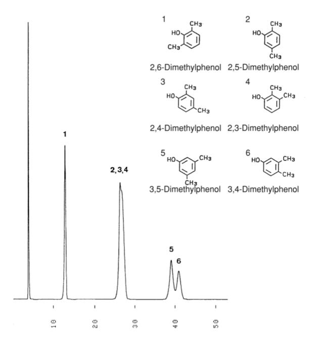
Column : YMC-Pack NH2 (5 μm, 12nm)
